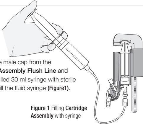
**Note:** Alternatively submerge the **Flush Line** in a basin of sterile saline. Pull back on the syringe plunger support until the fluid syringe is filled. Take care not to pull the plunger out of the syringe barrel.
