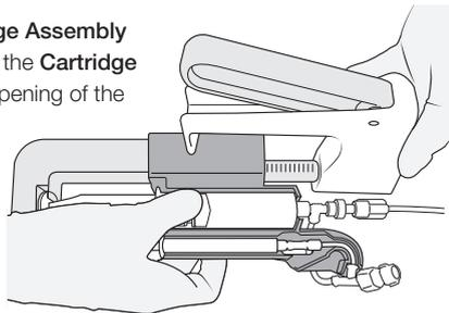
7. Remove the female cap from the **Microcatheter Connection Hub**. Before connecting the microcatheter, gently squeeze the **Control Handle** Lever to make contact between the **Microsphere Syringe** plunger and the **Cartridge Assembly**.
